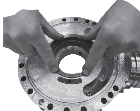
26. The outer surface of the side plate should be flush with the flange when pushed down. Once the push is removed the side plate will move out a little due to the o-ring below
