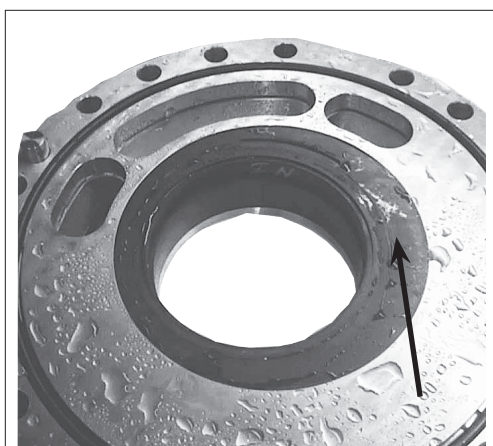
20. Position the sealing plate over the guide pin.
