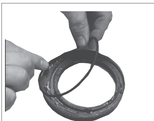
18. Assemble the new O-ring on the correct sealing plate. It is important to lubricate to ensure the O-ring does not drop out.
