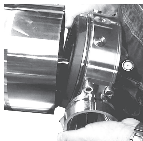
11. Carefully position the flange assembly onto the guide pin in the casing.
