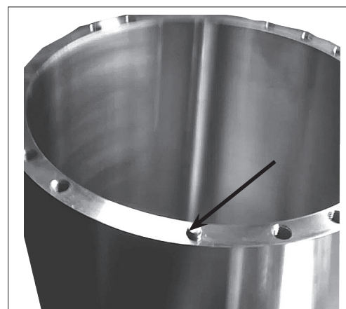
2. Position the guide pin into the casing.
