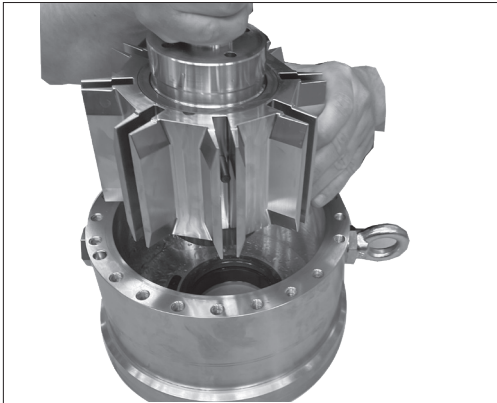
19. Carefully lower the rotor assembly into the housing. Taking care not to damage the side plate or the bearing. Spray the rotor with clean filtered water before installing the vanes.
