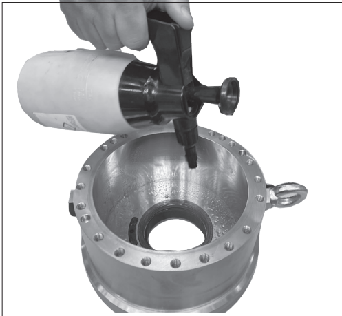
18. Spray the inside of the housing with clean filtered water before installing the rotor.
