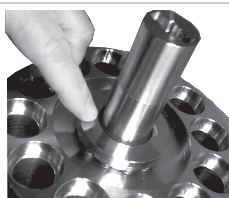
5. Carefully remove the tool assembly and check the O-ring assembly.
