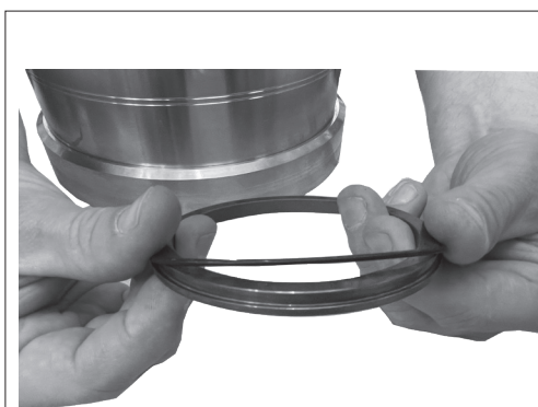
14. Install the O-ring on the rotor element.
