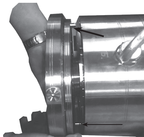
21. Carefully position the adapter flange assembly into the two guide pin holes.
