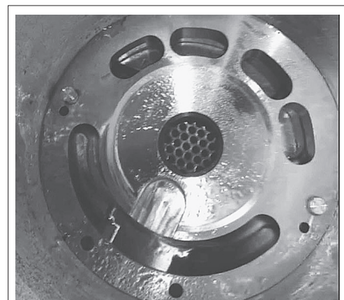
4. Turn the assembly and position the two guide pins in the flange inside the casing.
