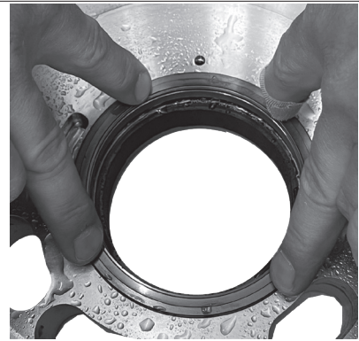
6. Carefully by hand press down the sideplate. The outer surface of the side plate should be flush with the flange when pushed down. Once the push is removed the sideplate will move out a little due to the oring below.
