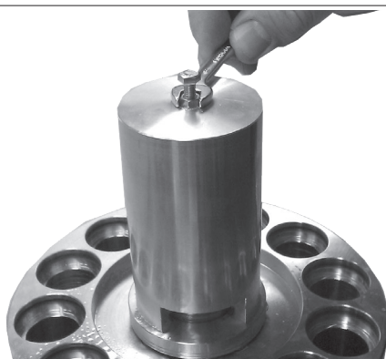
4. Using the tool provided, press down the retainer by tightening the nut until the O-ring is placed in the recess. If needed use a small screwdriver to get the O-ring into the recess.
