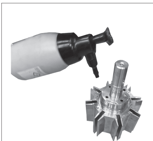
13. Place the rotor with the shaft pointing upwards and lubricate the grooves with water.
