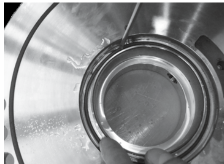
24. Mount the second new O-ring (pos. 137) in the bottom on the flange.
