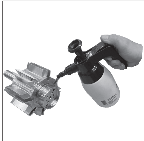
8. Place the rotor in a horizontal position and lubricate the end with water.
