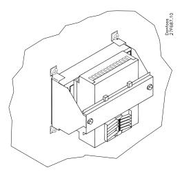
Install the front panel from outside of the electrical box.
