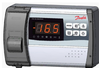
Fig 8. Close the front panel, making sure that all the wires are inside the box and that the box seal sits in its seat properly. Tighten the front panel using the 4 screws. Power up the panel and carry out thorough reading/programming of all the parameters.
