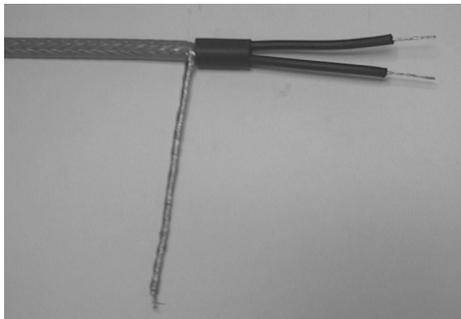
6. Crimp tube 9/3, L=20 mm is pulled in over the two conductors, all the way to the twisted screen in order to cover approx. 10 mm of the primary insulation and approx. 10 mm of the conductors.
