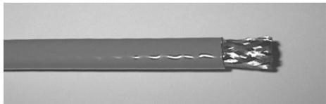
1. Remove 15 mm of the outer sheath. Remove the screen braid from the 15 mm stripped cable, too. Be careful not to damage the primary insulation.
