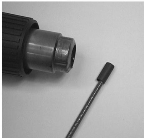
2. Crimp tube 6/2, L = 20 mm is pulled in over the end of the cable to the edge of the removed outer sheath. 5 mm of the crimp tube must still be free of the cable.
