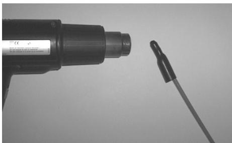
5. The end sealing is crimped down from the sealed end and in over the cable. Make sure that the glue is running out from the end of the end sealing.
