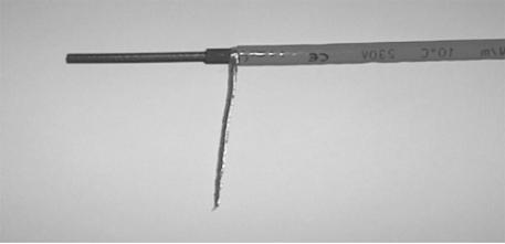
2. The screen is released and twisted. Following this, remove the outmost 80 mm of the primary insulation. Use knife.
