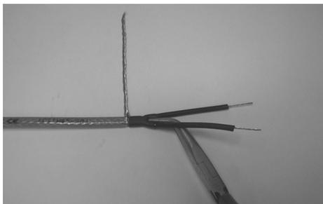
7. The crimp tube is crimped down and immediately after this the outmost 10 mm are squeezed together on the middle with flat pliers.
