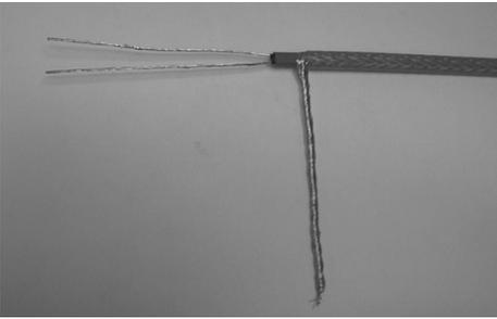
3. The core material is removed from the conductors, also from the outmost 80 mm. Be careful no to damage the conductors.
