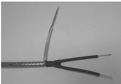
8. Yellow/Green, L=50 mm tube is pulled in over the twisted screen.
