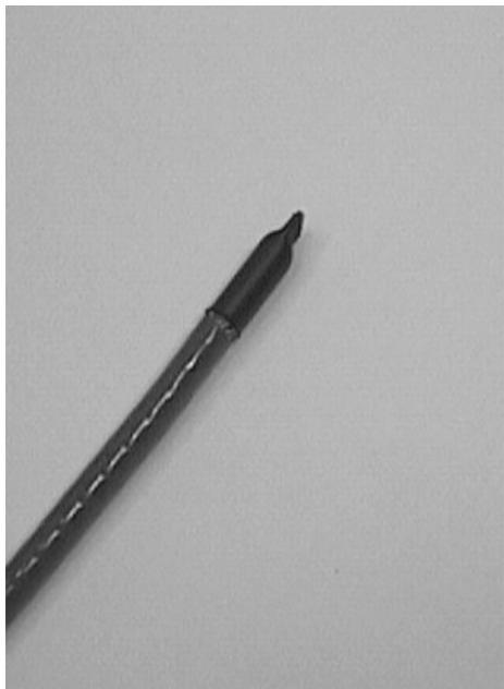
3. The crimp tube is crimped down, whereafter the outer 5 mm is squeezed with a pliers. Make sure that the glue is running out from both ends of the crimp tube.
