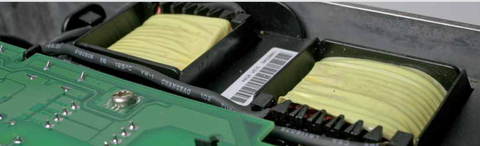
Built-in intermediate circuit coils reduce low-frequency mains feedback and increase the life of the drive.
