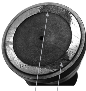
Abrasive wear of the piston shoes. All pistons must be replaced immediately.
