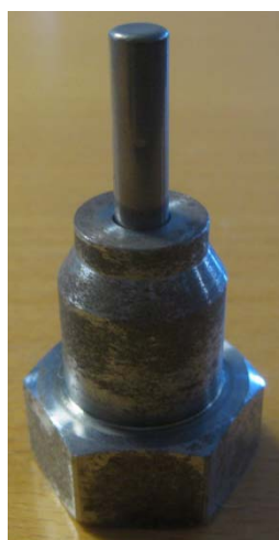
Present AKS 21W with Free cut steel bushing and press welding
