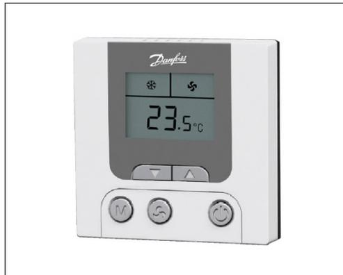
REPI series thermostats are used to control room temperature in industrial, commercial and residential environment via controlling electric modulating valve with 0-10VDC (4-20mA) control signal or floating control as well as damper actuator of VAV system.
