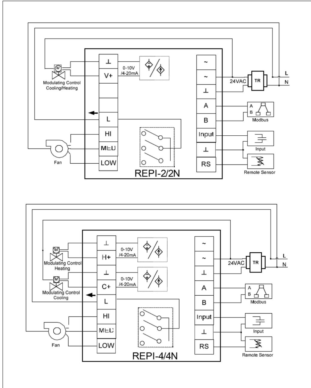
Note: Be sure to connect all the wires as per the wiring diagrams and keep it away from water, mud and other material so as to prevent the unit being spoiled!
